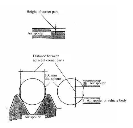
3. The following air spoiler which exhibits no damage, etc. shall be
