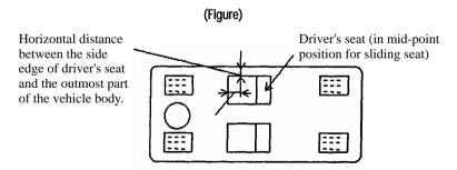
B. The surface of the section located at the side of the driver's seat and the seat which is parallel thereto and adjacent to the side of the motor vehicle is covered with impact-absorbing material and has no sharp projection.
