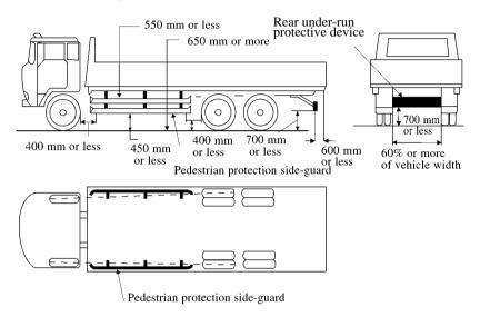
(4) The pedestrian protection side guard shall be mounted so that the flat section thereof is located outside of a straight line connecting the centres of the road contact sections of the outermost front wheel and outermost rear wheel, and the mounting section thereof is located 150 mm or more inside of the flat section.
