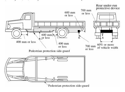
(Example 2) (Example of installation on large-sized truck with a gross vehicle weight of 8 tons or more, or with a maximum loading capacity of 5 tons or more)
